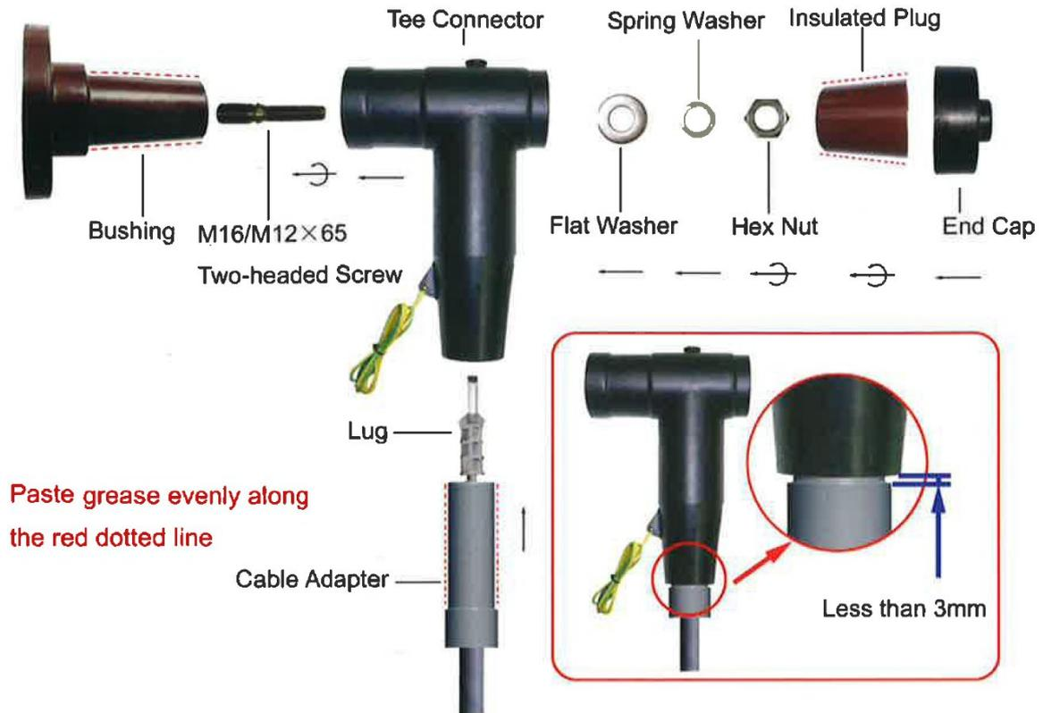
Figure 3- 17 Tee Connector Installation
