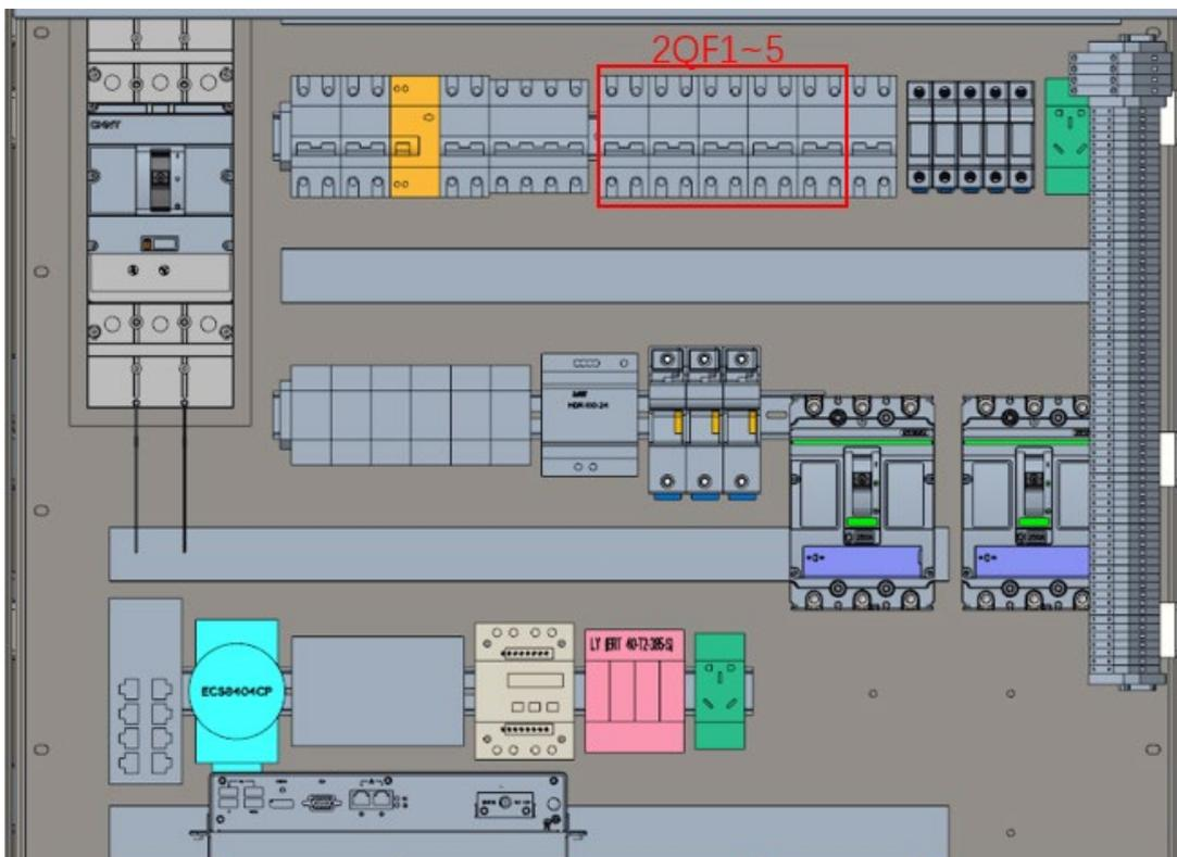
Figure 4- 2 Close 2QF1-2QF5 micro circuit breaker
